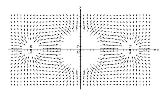
3. The figure above represents the electric field in the vicinity of three small charged objects, R, S, and T. The objects have charges -q, +2q, and -q, respectively, and are located on the x-axis at -d, 0, and d. Field vectors of very large magnitude are omitted for clarity.
