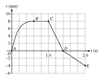
A cart is constrained to move along a straight line. A varying net force along the direction of motion is exerted on the cart. The cart's velocity  $\nu$  as a function of time t is shown in the graph above. The five labeled points divide the graph into four sections.
