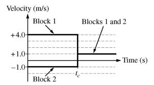
Block 1 of mass  $m_1$  and block 2 of mass  $m_2$  are sliding along the same line on a horizontal frictionless surface when they collide at time  $t_c$ . The graph above shows the velocities of the blocks as a function of time.
