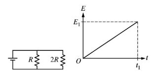
18. The circuit shown above contains two resistors of resistance *R* and 2*R*. The graph shows the total energy *E* dissipated by the smaller resistance as a function of time. Which of the following shows the corresponding graph for the larger resistance?
